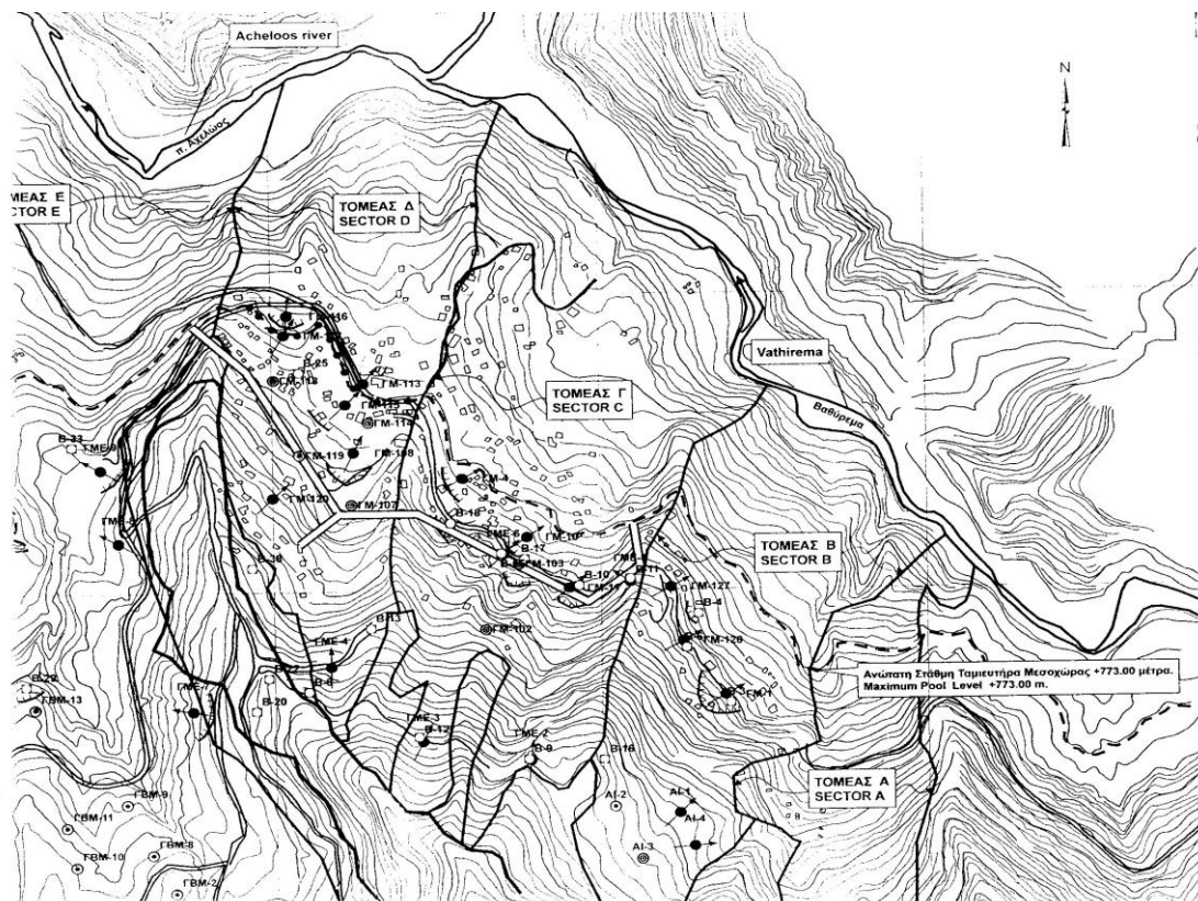
Figure 5. Mesochora village instrumentation-examined stabilization measures-scale 1:10000
