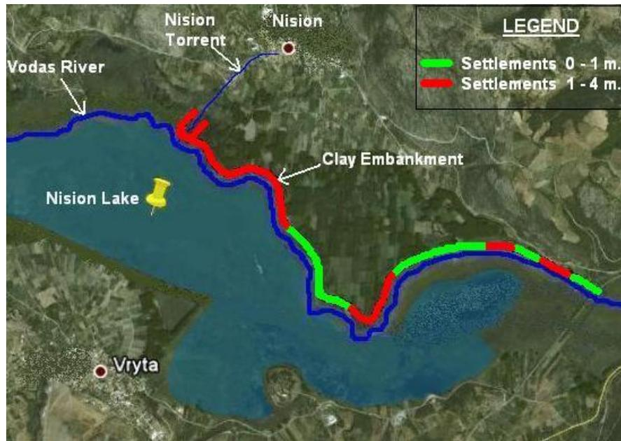
Fig.2 Twenty years observed settlements along clay embankment.
